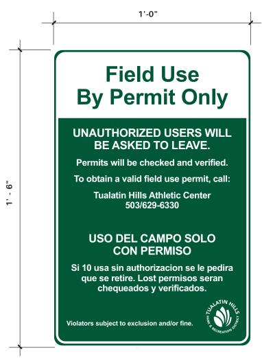
1 Elevation - Sign Type F1 F1.1 Scale: 3" - 1' - 0"
