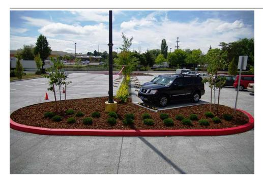
by: SUBMITTED PHOTO - New native plantings in linear tree wells work with the newly installed porous concrete pavement at Sunset Swim Center to filter and minimize stormwater runoff.
