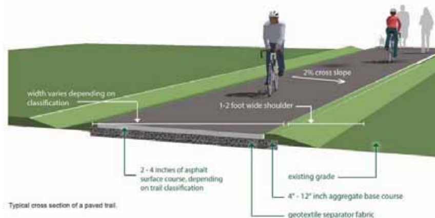
Figure 4F – Typical asphalt trail cross-section.
