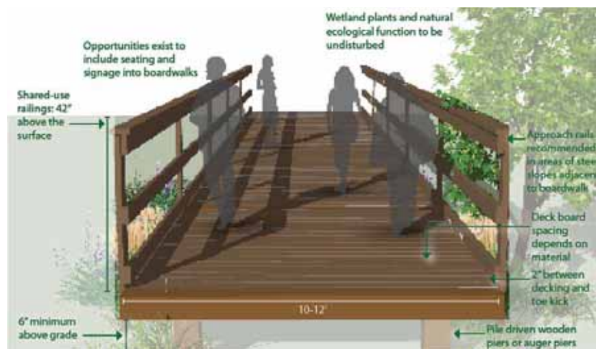
Figure 4G – Typical bridge/boardwalk cross-section.
