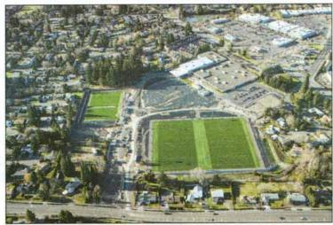
Plus, all playing fields needed to be level. That was a significant engineering challenge because the site's north side is 27 feet higher than its south side. Crews moved more than 50,000 cubic yards of dirt from one end of the site to the other.
